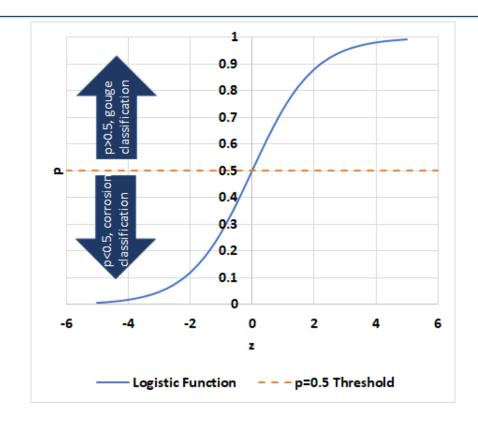
Inputs used – pipe geometry, ML clock location axial and circumferential distance of ML from dent center ML aspect ratio and dent strain
