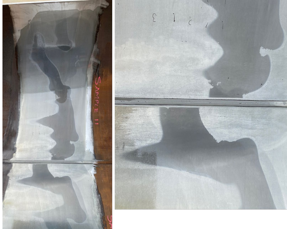
CMAs revealed from ID etching, corresponds to item a) saw tooth pattern in ID. Pattern discontinuous across seam weld.
