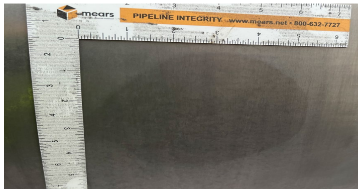
ECT Scan and Etching of AO Smith Pipe Body Hard Spot (338HB).
