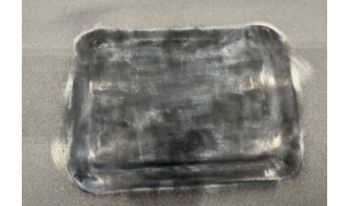
8-inch (l) x 1-inch (w), 45% or 85% deep groove corrosion feature
