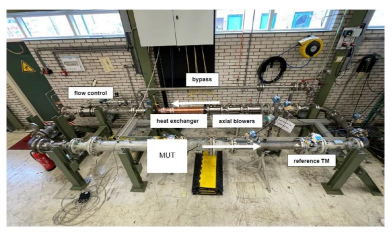
The first tests with hydrogen of the usual flow meters for custody transfer of natural gas
