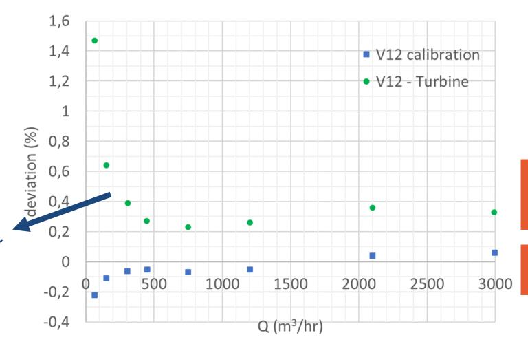
Baseline curve determined for deviation of Turbine vs. V12 on natural gas
