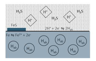
3 - 5 ppm-w H (measured for 1 bar H<sub>2</sub>S, pH3)
