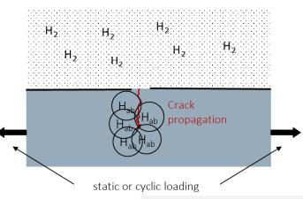
influence on ductility, crack propagation, fracture toughness, fatigue properties
