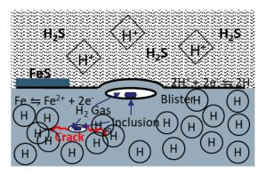
hydrogen induced cracking (HIC) or sulfide stress cracking (SSC)
