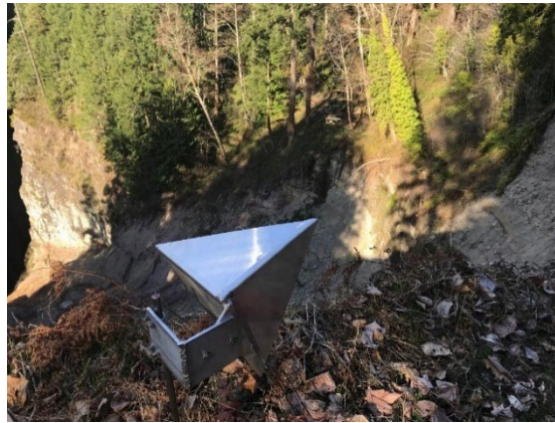
Figure 7 - Corner Reflectors on a slope that is being monitored with GBInSAR
