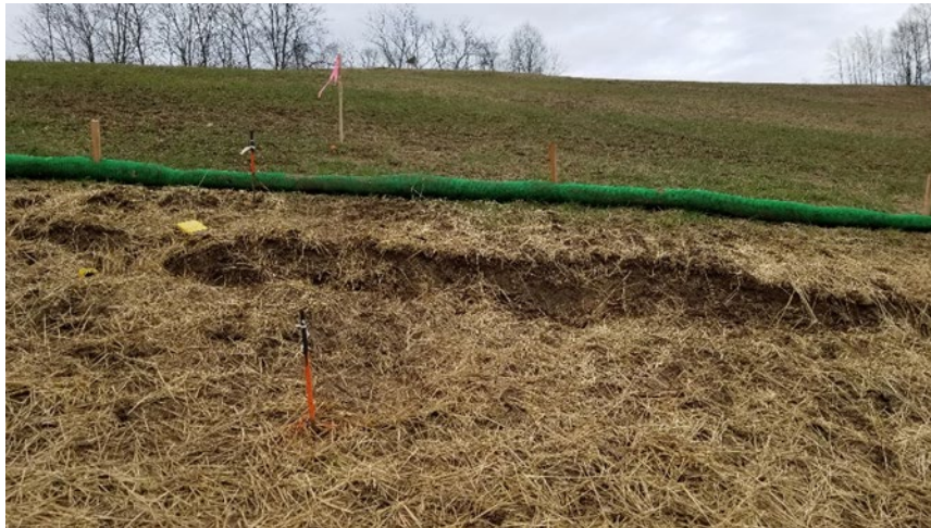
Figure 14 - Photo of Extensometer 300AB across tension crack
