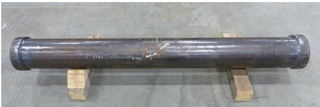
Figure 4 – Capped-end burst test specimen
