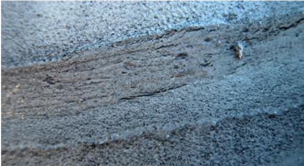
Figure 9: Crack in the gouge of damage BG2 from Pipe 1.
