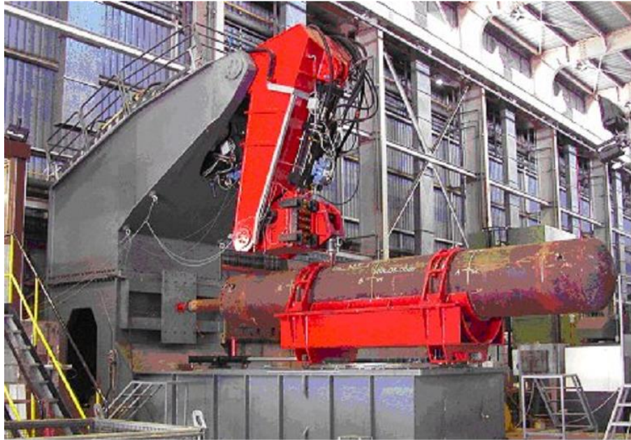
Figure 2: View of the RINA-CSM's full scale external damage testing facility (Simulator).
