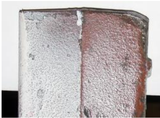
Figure 3: 33 tons excavator tooth: new (left) and worn (right).
