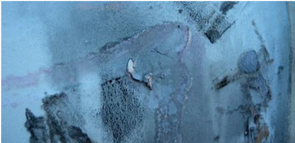
Figure 11: Crack in the gouge of damage G1 from Pipe 1.
