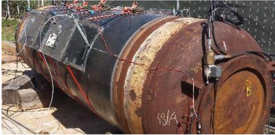
Figure 8: Pipe with cells ready for environment full scale test.
