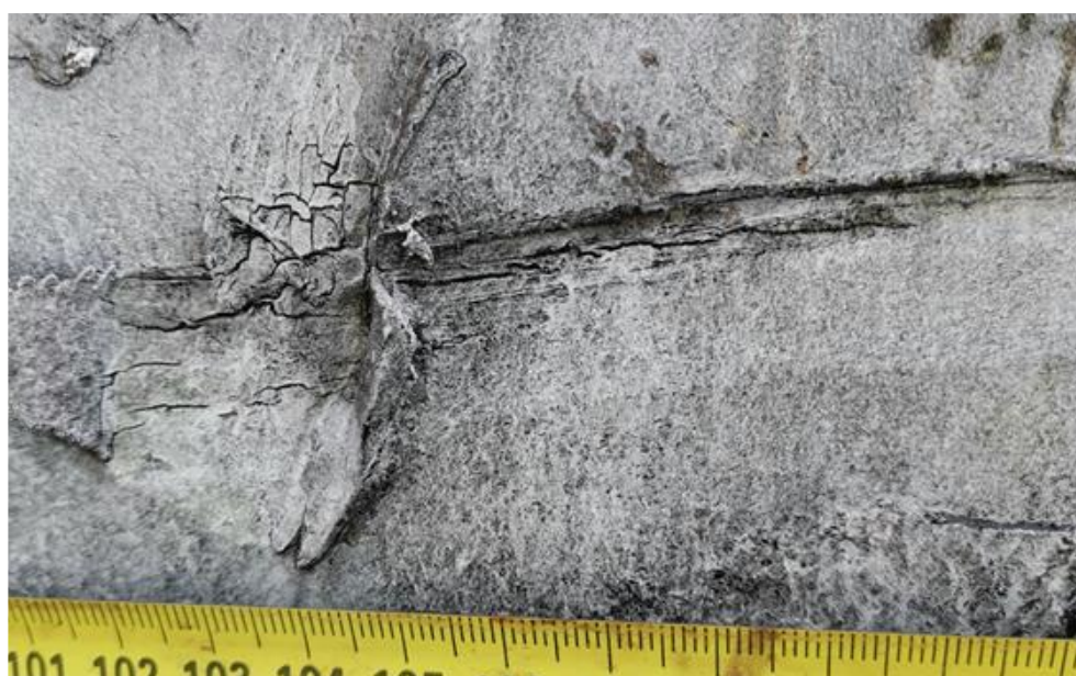
Figure 6: Cracks after damage creation.
