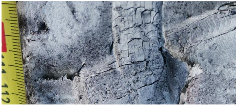
Figure 17: Cracks at end of gouge of damage BG2 from Pipe 5.
