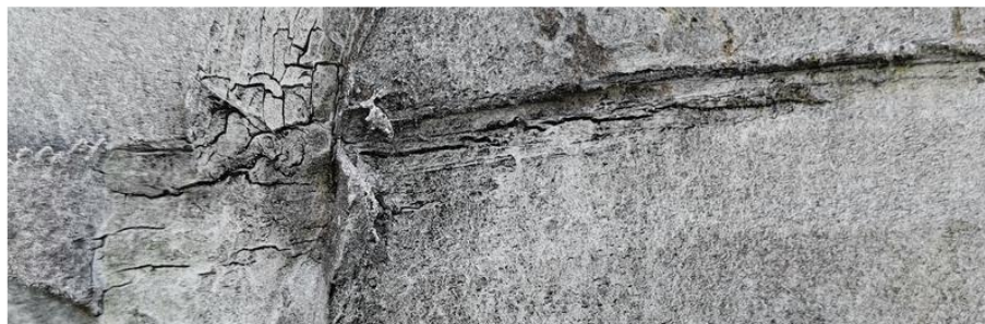
Figure 19: Cracks at end of gouge of damage BG4 from Pipe 5.
