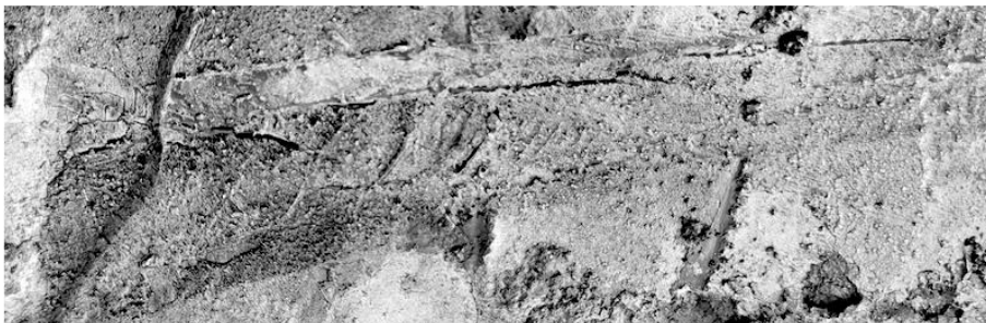
Figure 15: Crack in the gouge of damage BG1 from Pipe 5.
