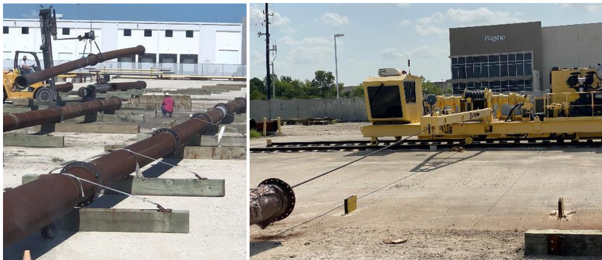
Figure 9: ILI Trial Setup and Pull Through Winch
