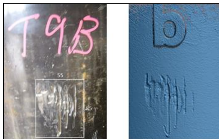
Figure 9: Example of Pipe damage and scanned image
