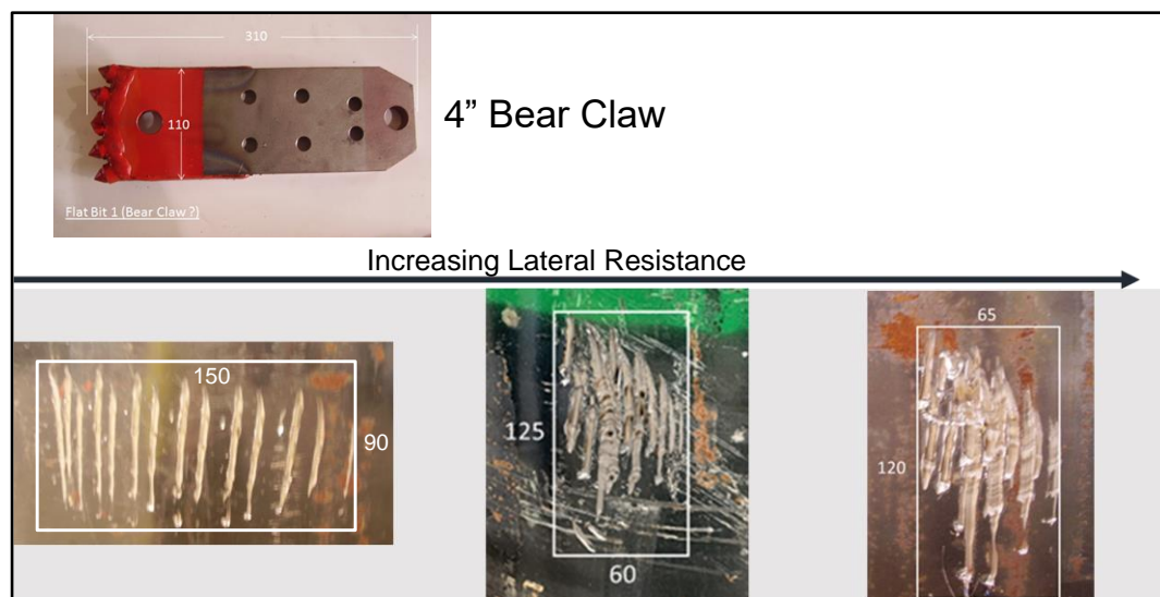
Figure 12: Pipe Damage 4" Bear Claw
