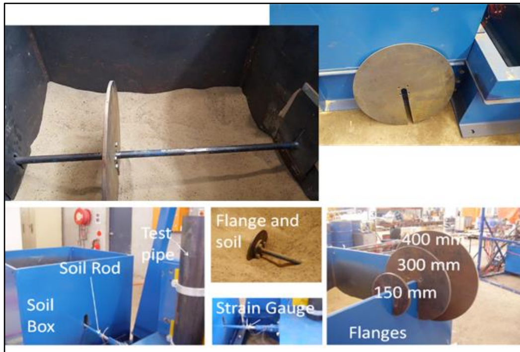
Figure 6 Soil Box, Soil Rod and Accessories
