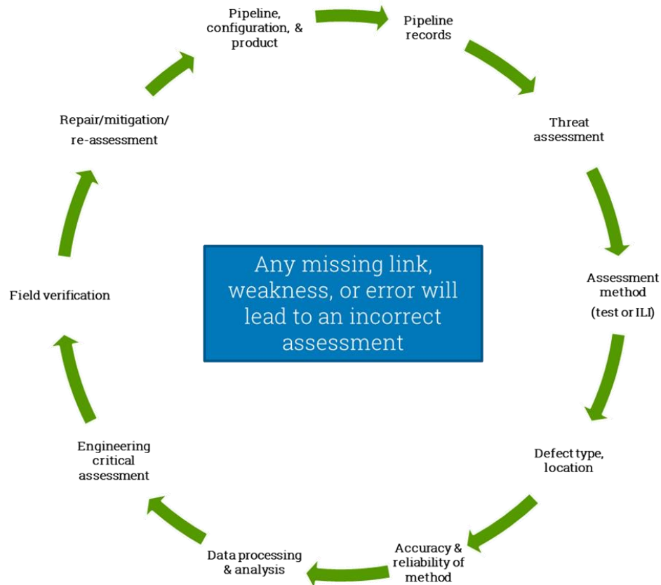
Figure 8 The crack assessment process
