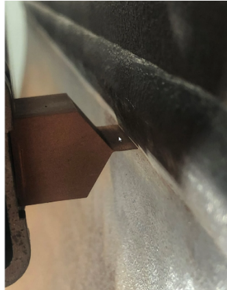
Figure 5: Notching of the seam weld at the weld toe during trials
