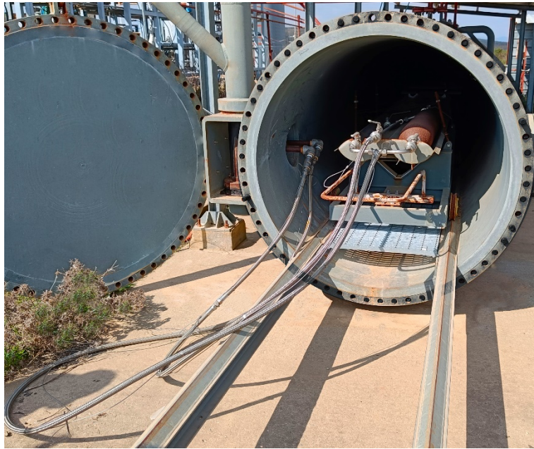
Figure 2- Example photo of a test vessel inside the safety chamber
