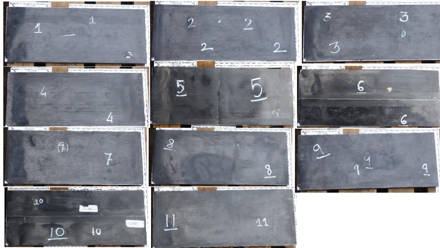
Plates surfaces were glued with 1mm thick black opaque ABS sheets
